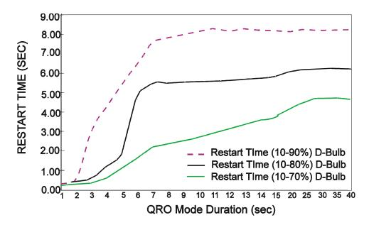
Figure 16. Restart Time Versus QRO State Duration, D-bulb
